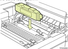
Install the fuser cleaner. When installing, the roller should be facing toward you.
