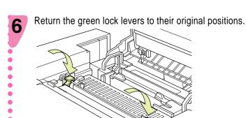
$\Box$  Do not return lock levers with force. If you cannot lock them easily, remove the photoconductor unit from the printer. Then re-insert it again until the gears mesh securely. After that, try again to return the levers to their original positions.
