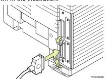
Attach the other end of the interface cable to the interface connector of the computer. Secure the cable.
