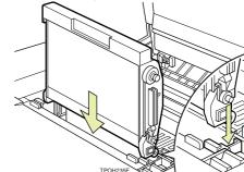
$\hfill\square$  When inserting the photoconductor unit, be careful not to touch or damege the surface.
