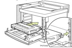
$\square$  Do not use excessive force in sliding in the cartridge.
