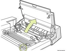
Remove the orange lock pins.
