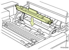
Turn the lock levers to hold the oil bottle and fuser cleaner.
